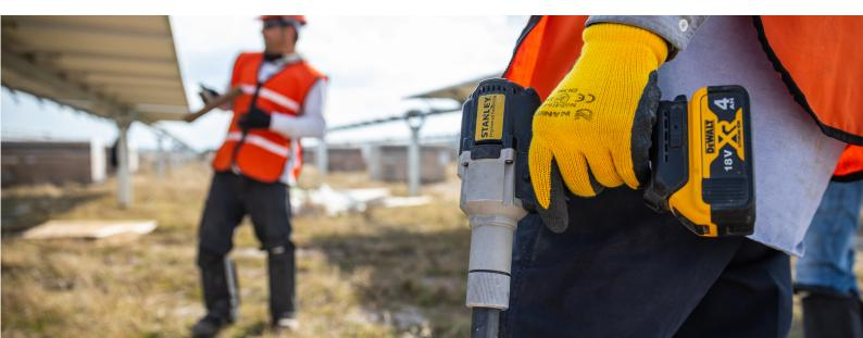
tools offer improved ergonomics, allowing users to maneuver in all directions without having to "fight" with air hoses to do their jobs. Data from a McMaster University study<sup>8</sup> comparing battery-operated and pneumatic tools suggests that the use of cordless tools reduces the demands on the forearms during use.
