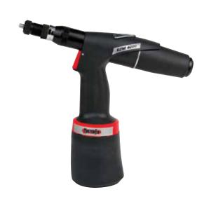
Light weight hydraulic/pneumatic blind rivet nut tool. Mandrels, M4-M8. Tool-free stroke setting mechanism with a scale on the front sleeve. Quick mandrel release system, Advanced hydraulic system for oil free service. Release button for motor release and 360° revolvable air supply unit.
