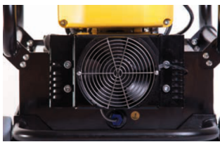
Reservoir heat exchanger
