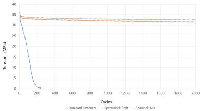
Spectralock design was proven to have superior vibration loosening resistance and performance.
